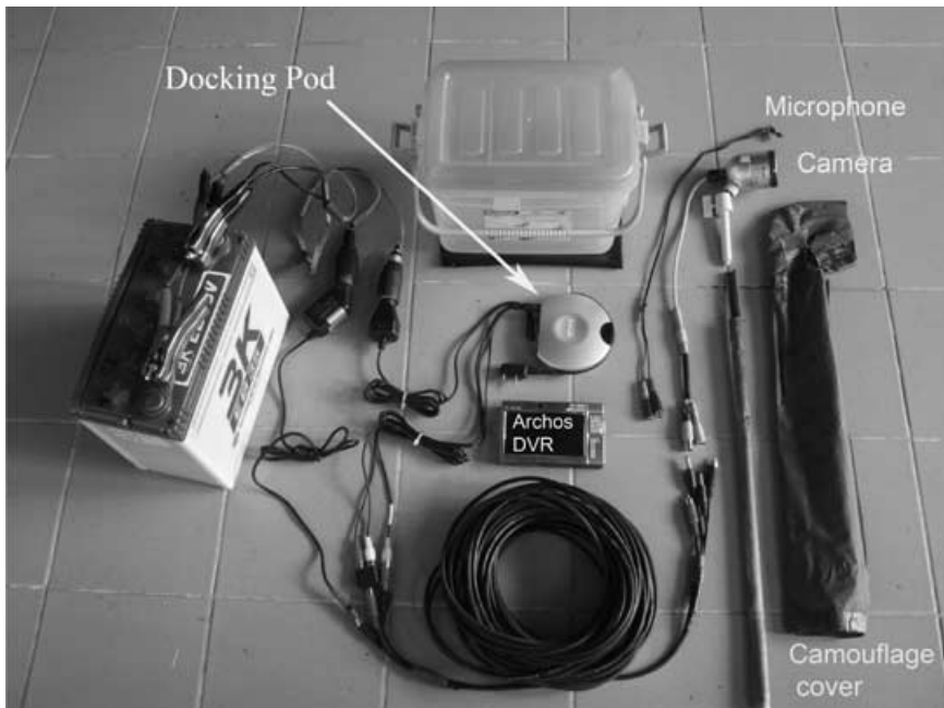
Fig. 1. Individual components of the video surveillance system.
